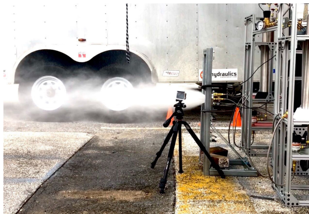
↑ A successful flow test using water provides key data to characterize the custom-designed engine and nozzle.
